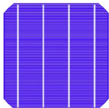
G-II: Four-busbar solar cell design (busbar width = 1.125 mm)
