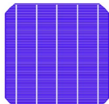
G-III: Five-busbar solar cell design (busbar width = 0.9 mm)
